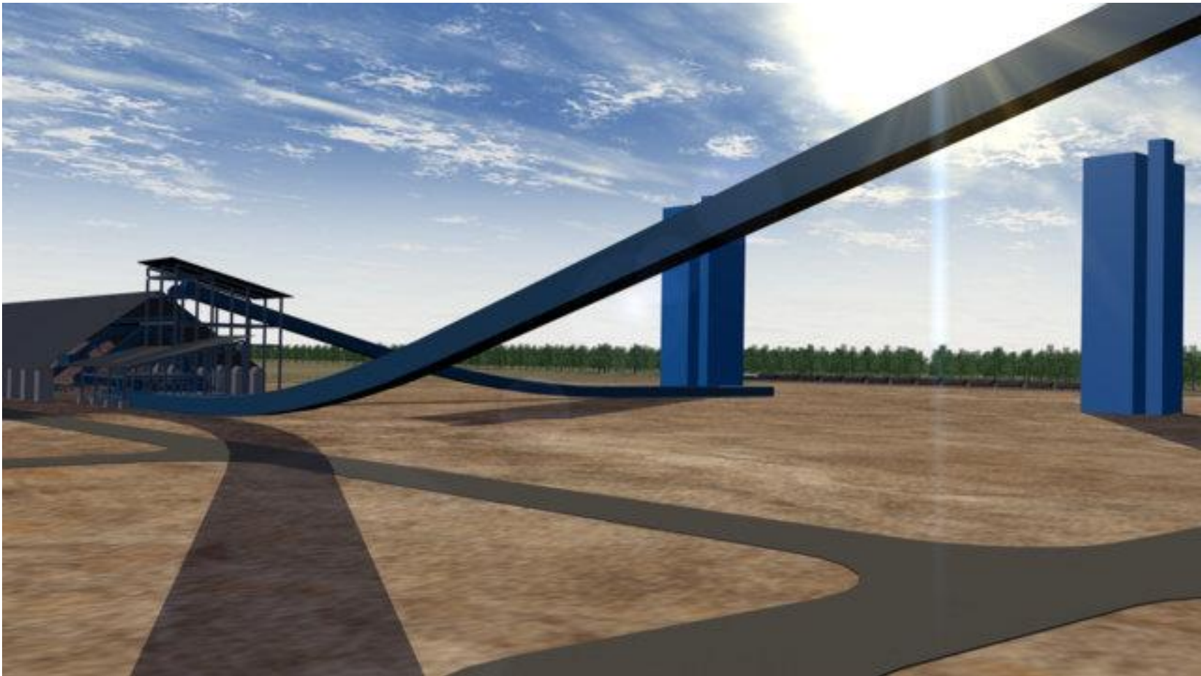
Figure 12: NAP-Foam Lake Plant looking southeast showing production shaft, conveyance to raw ore storage building and conveyor gallery to mill. The service shaft for manpower and supplies is located on the right.
